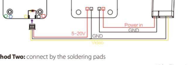
**Method Two:** connect by the soldering pads
