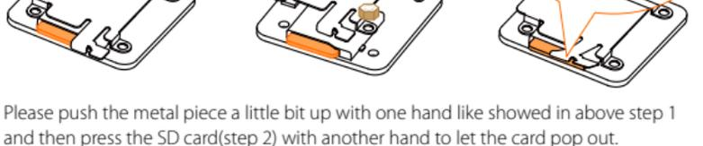
Please push the metal piece a little bit up with one hand like showed in above step 1 and then press the SD card(step 2) with another hand to let the card pop out.
