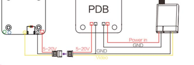
**Warning:** Current Input  $\geq 1A$  (Don't powered by VTx)
